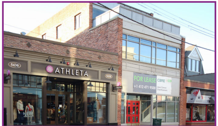
To Create a Cohesive Commercial District, Use Setbacks on Upper Floors to Diminish the Visual Size of the Building
